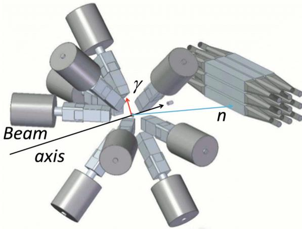
**Fig. 1.** Schematic diagram of the experimental setup. The AFRODITE  $\gamma$ -ray spectrometer consists of 9 HPGe clover detectors in BGO shields, 5 were at  $\theta_{\text{lab}} = 90^\circ$  and 4 at  $\theta_{\text{lab}} = 135^\circ$  with respect to the beam direction. The neutron detectors were arranged in three walls of three detectors placed at  $0^\circ$ .
