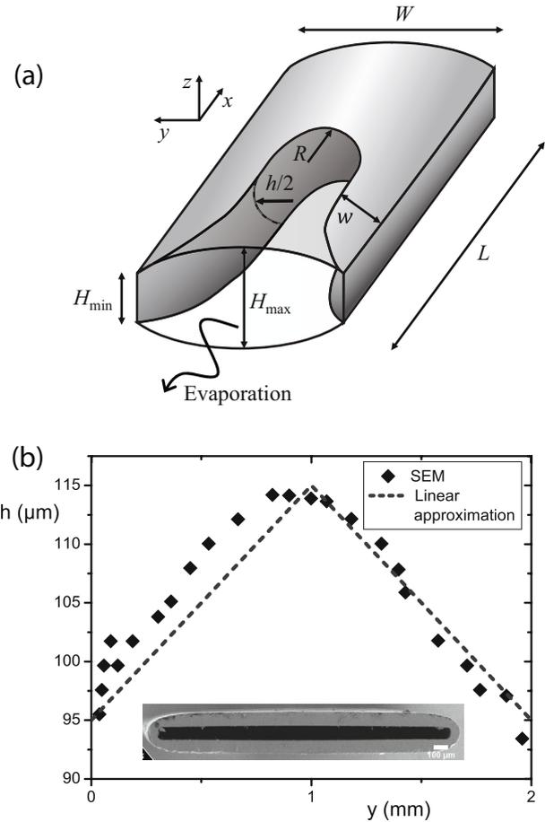
**Fig. 1.** Schematic of the experimental geometry: a glass channel with rectangular-like cross section closed at one end and at the entrance open for evaporation. The receding air/water interface is qualitatively sketched. (b) Channel height,  $h$ , measured from the SEM images of our geometry a function of the transverse position,  $y$ . The linear approximation is used for modeling (dash line).
