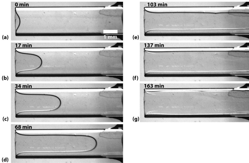
**Fig. 3.** Top views of the channel (open on the left) at different times during drying: (a) initial and after 17 (b), 34 (c), 68 (d), 103 (e), 137 (f) and 163 min (g). The scale bar denotes 1 mm and applies to all panels.
